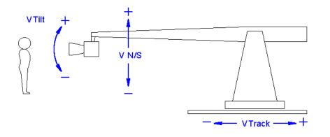
Vtrack Virtual Track; Calibrated in real-world centimeters. Vtrack is roughly analogous to the depth axis in a typical CG setup. Note that Vtrack *increases* moving out *away* from the set, and *decreases* moving in *toward* the set, this may be counter-intuitive to many operators. Zero is arbitrary.
